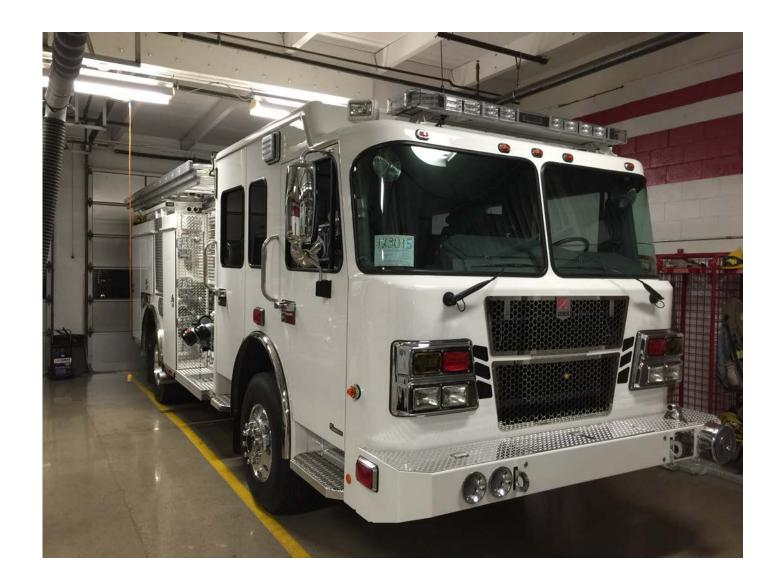
After final delivery, the long process of getting the engine ready to place in service began. Tasks included; striping, electronics install, compartment fabrication, DMV registration, and tool mounting just to name a few. This all took place by the Station personnel while still maintaining the daily operations of a Fire Department. The process took longer than expected, however the final product was exceptional.
