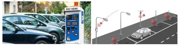
**Pros:** Pay with credit/debit card or use Season Pass barcode scanner/fob. Does not require staffing to operate. One or more can be placed in specific areas for customer access. No gates or in ground traffic spikes needed.
